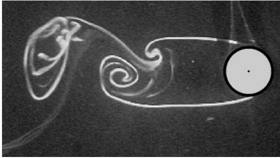
Figure 3. Image showing the visualized vortex formation region behind the stationary cylinder, when the 'lower' vortex is fully formed.
